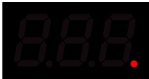
Display when the active mode is activated (<1 sec. pressing of the start button) and during the measuring process.
