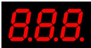
Display when measuring mode is activated (>1 sec. pressing of the start button)
