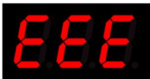
Display of an "Error", e.g. due to an operating error during the measurement process or a full measurement data storage.
