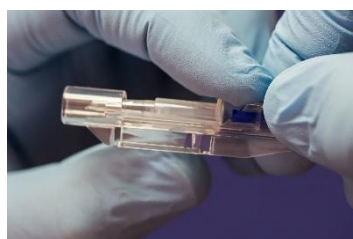
b) Careful mount the nozzle on the hand-piece as shown above.
