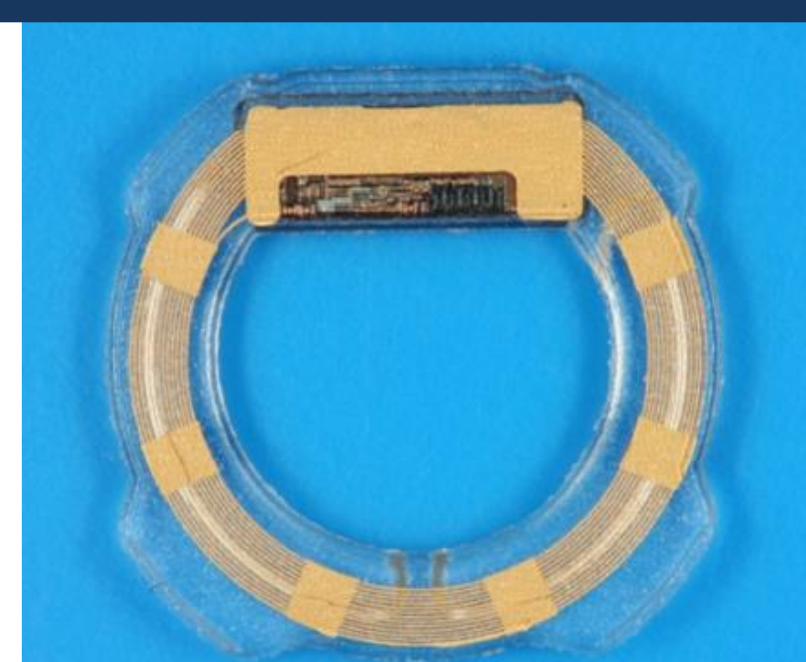
1 EYEMATE™ sensor. Implantation during cataract surgery in the ciliary sulcus, in front of the intraocular lens.
